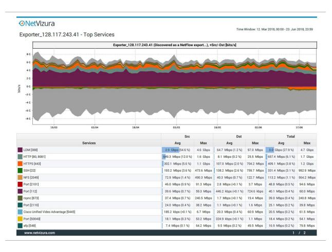
Cluster real server backends and accumulator nodes routinely have instantaneous output volumes that approach 2 Gbps. Bonding of pairs of gigabit Ethernet interfaces was needed to be able to support these output data rates. The next generation of cluster machines to be installed soon will have 10 Gbps Ethernet capability.
