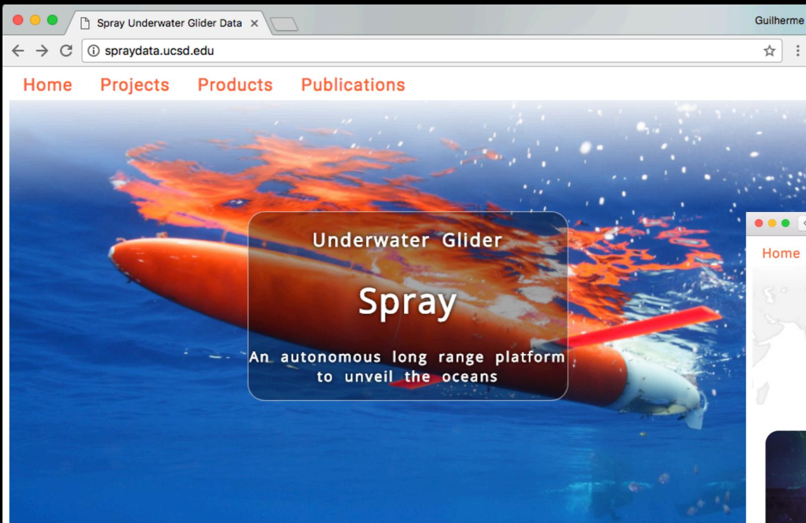
Underwater gliders are autonomous vehicles that profile vertically by controlling buoyancy and move horizontally on wings. Russ Davis, Jeff Sherman and the Instrument Development Group at Scripps Institution of Oceanography have developed the glider Spray. Spray is 2 m long and weighs 50 kg. It communicates to shore using Iridium, and navigates with GPS. Spray steers by changing its center of mass through the movement of
